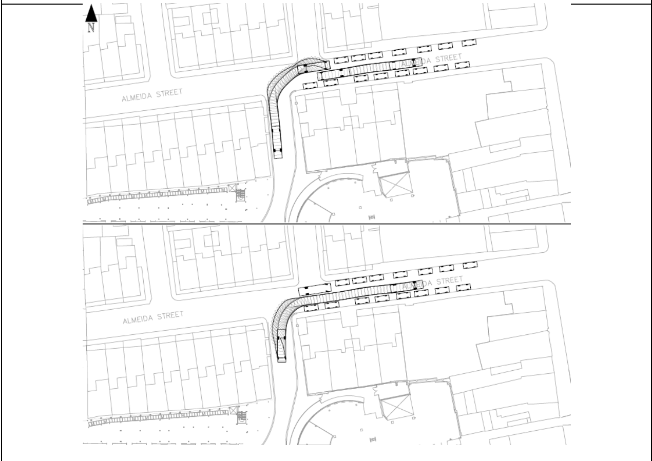
Figure 11: Swept path vehicle tracking for a 10m rigid van at the Almeida Street access and negotiating parking bays on Almeida Street.
